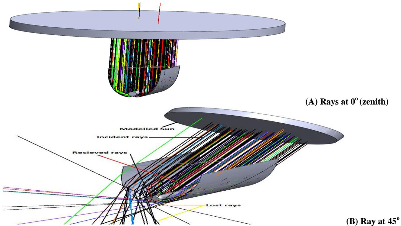
**Figure 3:** Trajectories of the rays incident on CPC at different solar hour angles
