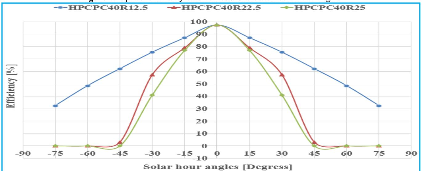
Figure 5: Optical efficiency of HPCPC40 at different solar hour angles
