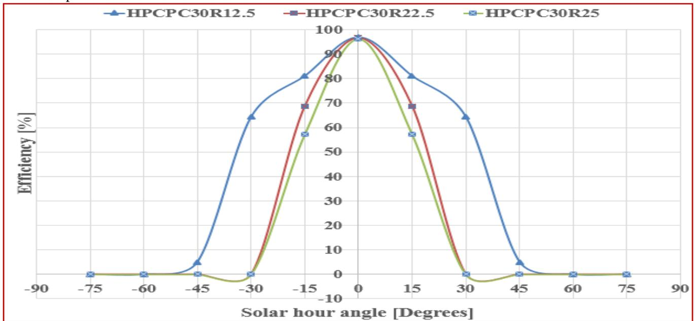
Figure 4: Optical efficiency of HPCPC30 at different solar hour angles
