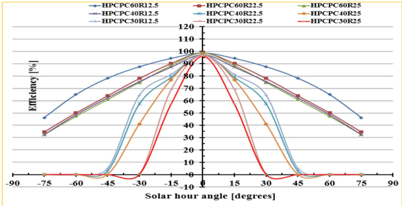
Figure 8: Optical performances of HPCPC configurations at different incident angles
