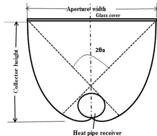
Figure 1: Compound Parabolic Collector
