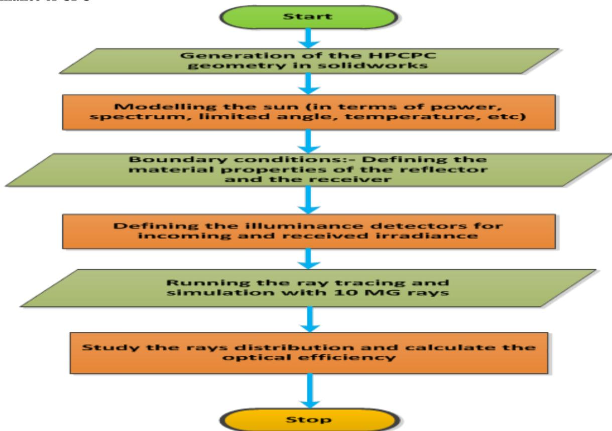
Figure 2: Flow chart of the modelling process of HPCPC using ray tracing technique
