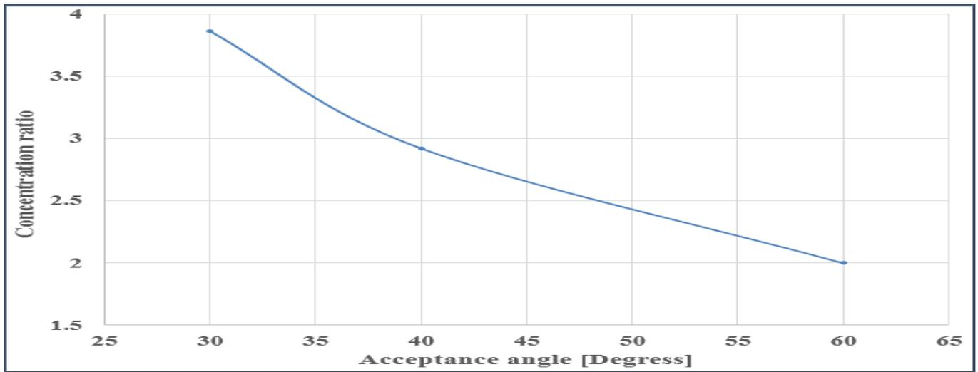
Figure 7: Variation of concentration ratio with the acceptance angle
