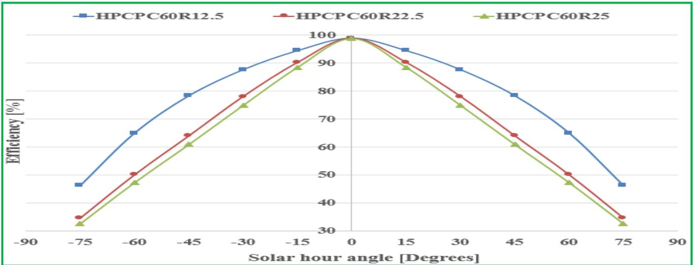
Figure 6: Optical efficiency of HPCPC60 at different solar hour angles
