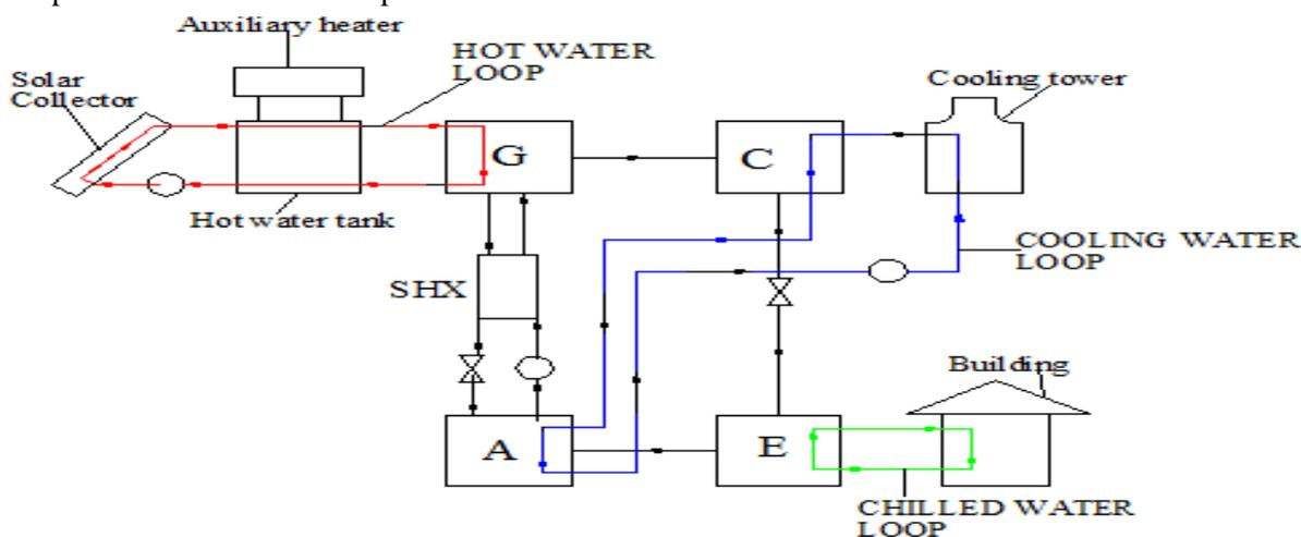
Fig. 3: Schematic of SAC system (G: generator, C: condenser, E: evaporator, A: absorber, SHX: solution heat exchanger)
