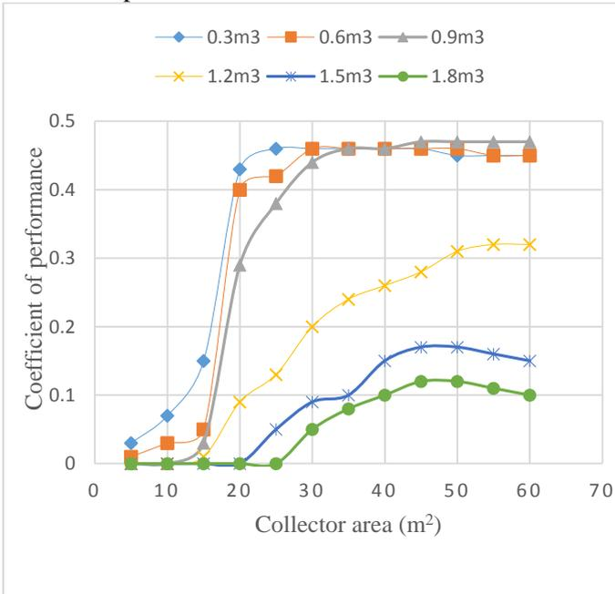
Fig. 7: Variation of coefficient of performance with collector area and hot water tank storage volume for the month of August.
