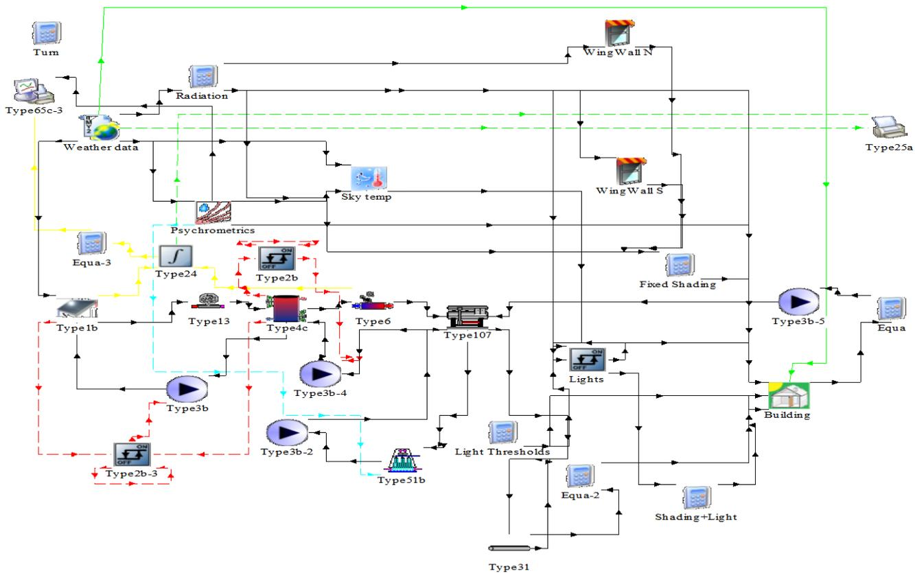
Fig. 4: Model of the SAC system in TRNSYS studio
