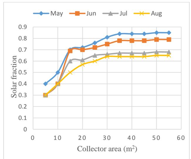
Fig. 9: Variation of solar fraction with collector area for the months of May to August.
