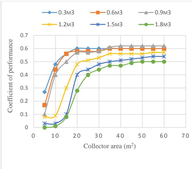
Fig. 6: Variation of coefficient of performance with collector area and hot water tank storage volume for the month of April.
