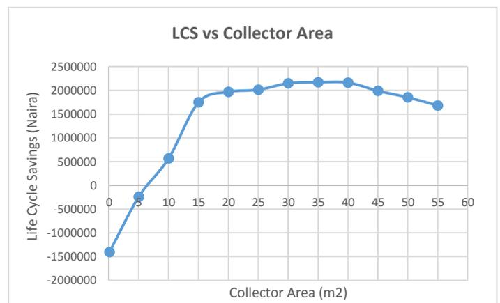
Fig. 13: Variation of life cycle savings with collector area.
