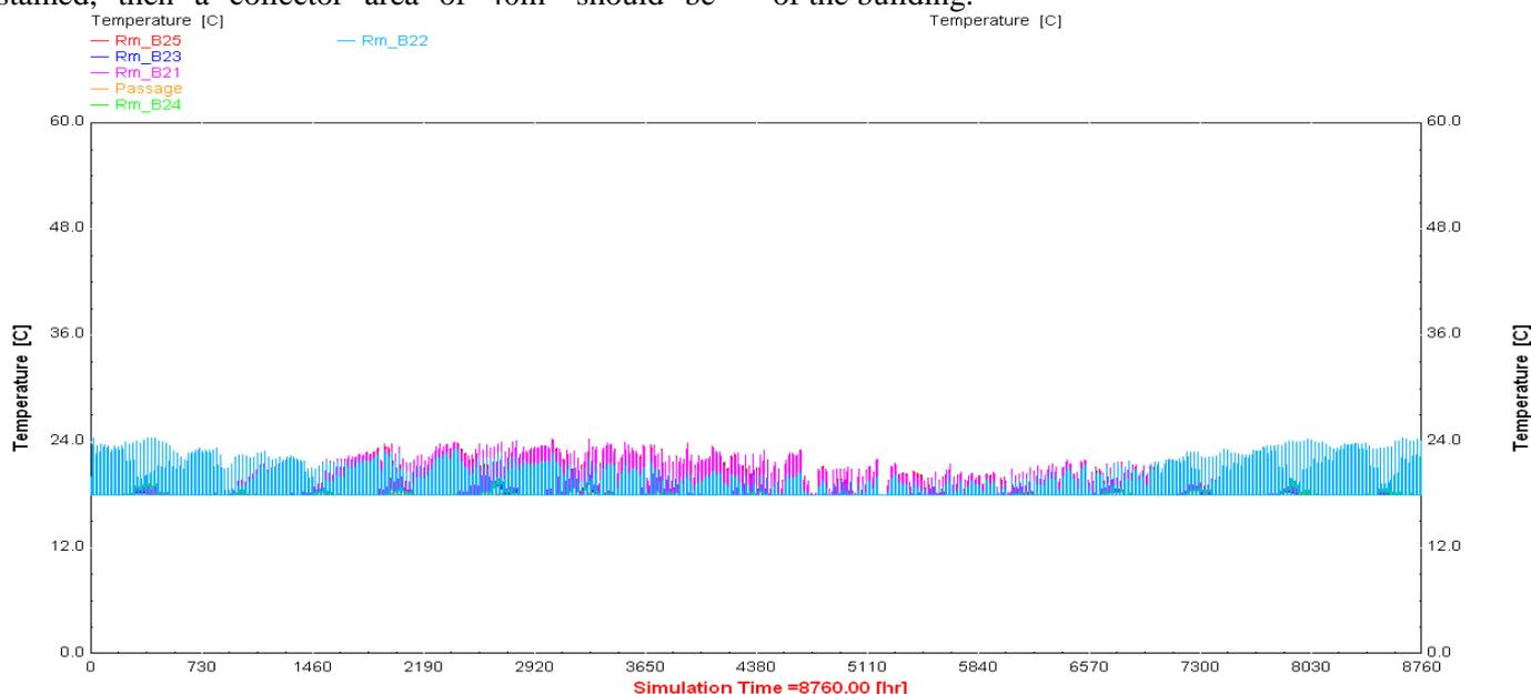
Fig. 14: Temperature variation within the zones for the whole year with cooling from the optimized SAC system.
