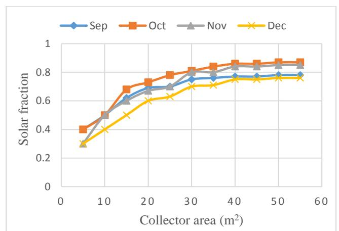
Fig. 10: Variation of solar fraction with collector area for the months of September to December.
