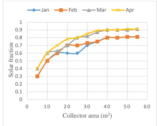
Fig. 8: Variation of solar fraction with collector area for the months of January to April.
