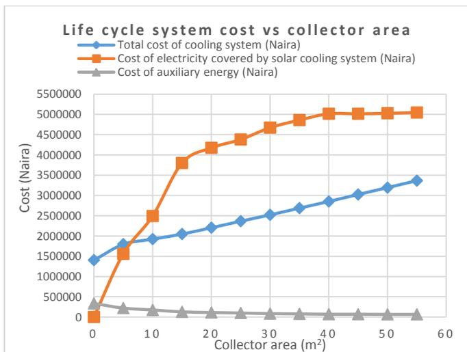
Fig. 12: Variation of total cost of cooling system, cost of electricity covered by solar cooling system and cost of auxiliary energy with collector area.
