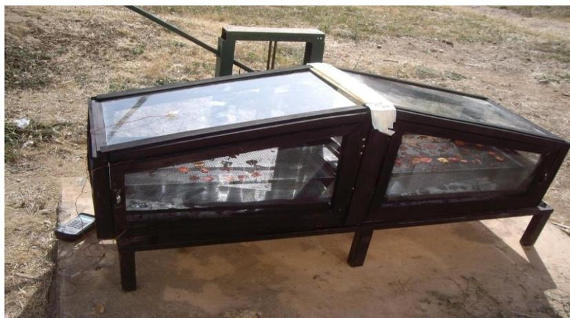
**Fig. 1: Pictorial view of the developed double compartment solar dryer during test**
