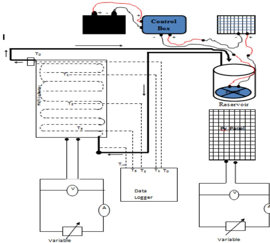
Fig. 2: Experimental setup for investigating the effect of cooling on temperature coefficient of PV module
