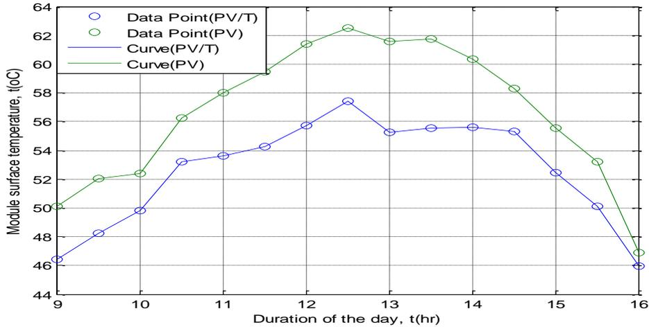
Fig. 5: Effect of cooling on PV module surface temperature
