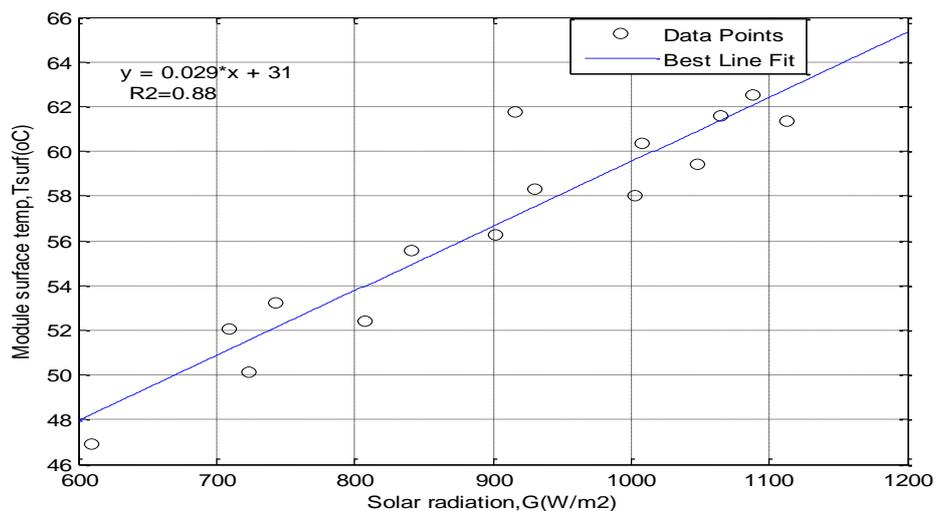
Fig. 4: Solar radiation - solar PV module temperature interaction
