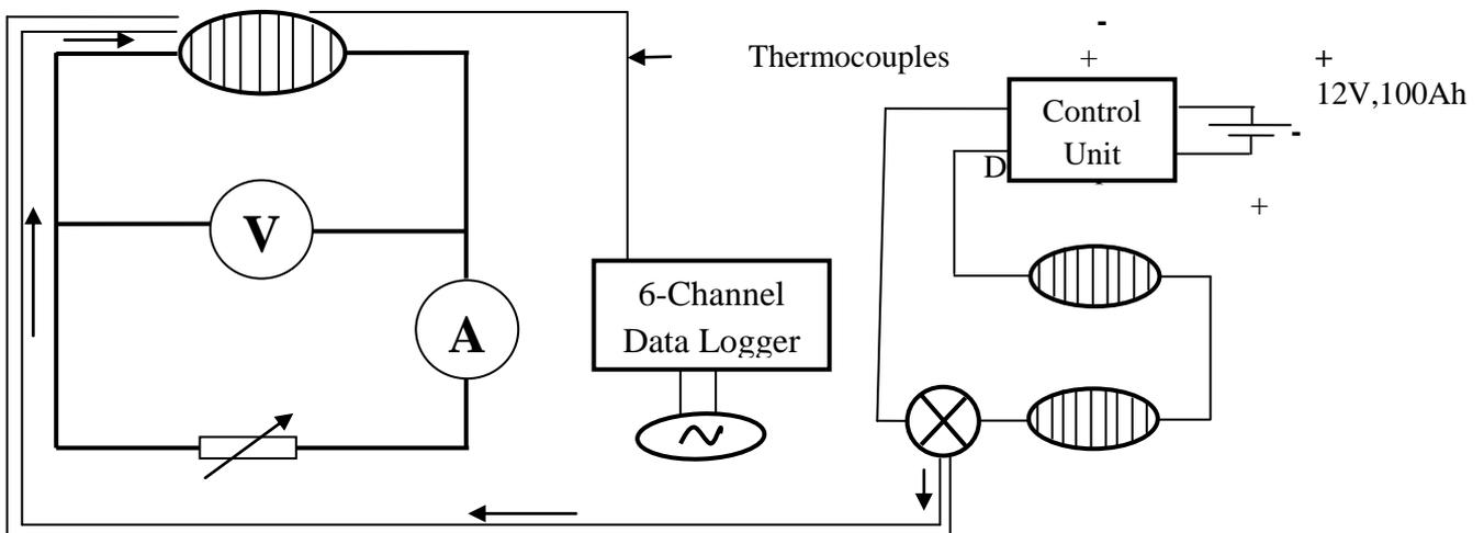
Fig. 3: Equivalent circuit diagram for investigating the effect of cooling on temperature coefficients of PV modules
