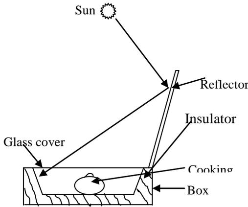
Fig. 1: Sectional View of the Solar Box Water Heater
