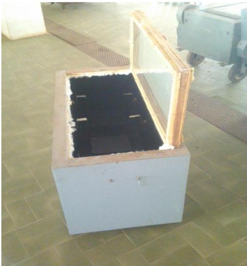
Fig 2: Picture View of the Solar Box Water Heater
