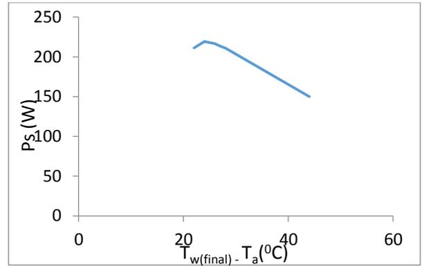
Fig. 4: Standard Effective Power versus Temperature Difference Plot
