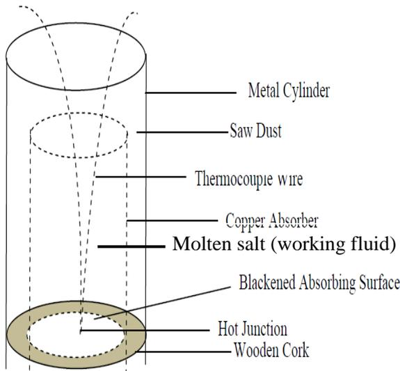
Fig 3. The solar radiation absorber.
