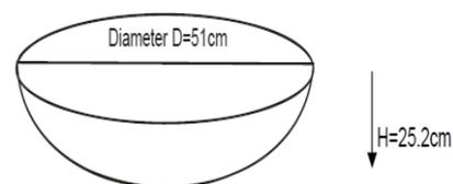
Fig. 1: Hemispherical Paper Mould
