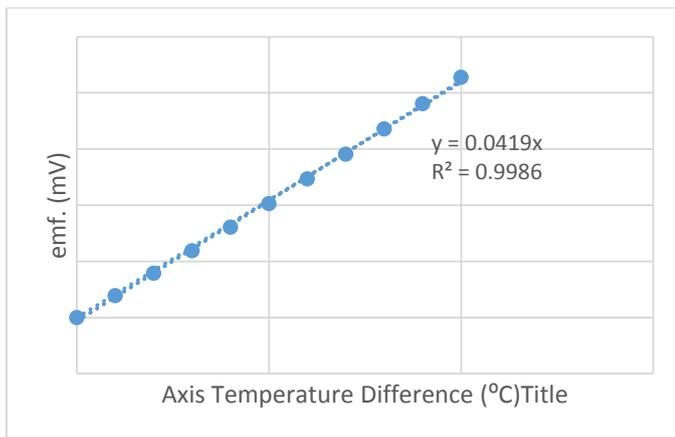
Fig. 5: Calibration Curve of Copper – Constantan Thermocouple (Handbook of Chemistry and Physics, 59<sup>th</sup> Edition).
