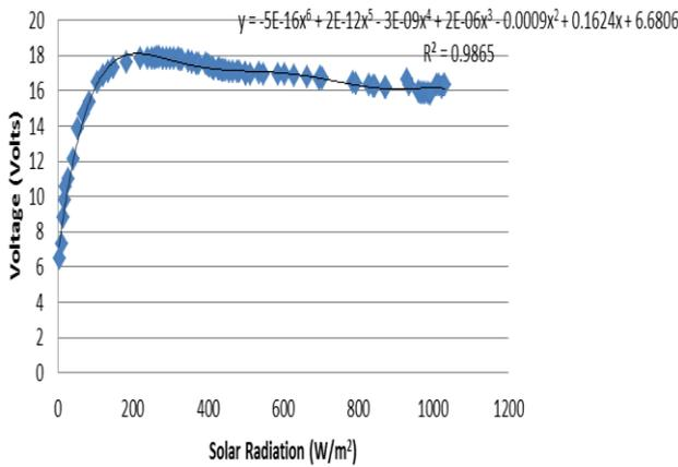
Fig. 5: Graph of solar cell incident radiation against voltage
