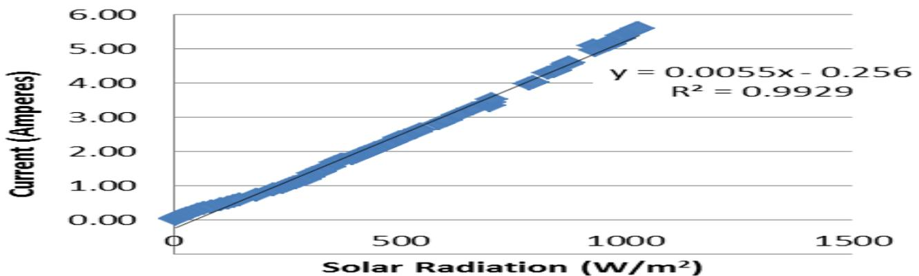
Fig. 4: Graph of Solar Cell Short Circuit Current Test
