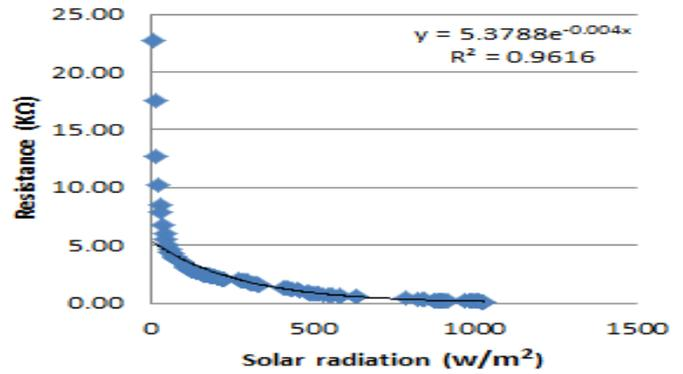
Fig. 3: Graph Of LDR Incident Solar Radiation against Its Resistance  $m^2$
