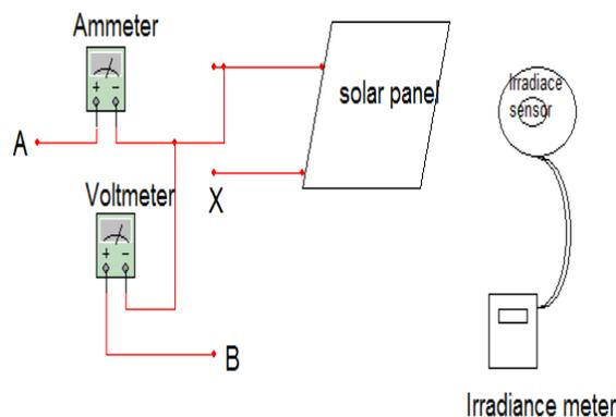
Fig. 2: Solar Cell Experimental Set-up
