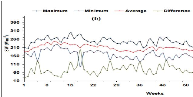
Fig. 1b: Weekly average SW (Wm-2) Plots of maximum, Average, Minimum, and Difference between Maximum and Minimum (in that order from top to bottom) compared over the solar cycle
