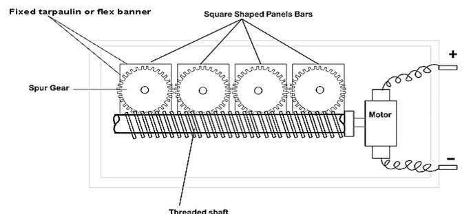
Fig. 12: Sectional View of the Spur Gear, Threaded Screw Roller and Square-Shaped Display Panel Bars.
