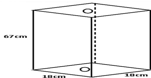
Fig. 11: Isometric View of the Square-Shaped Display Panel Bar
