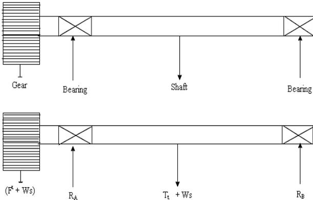
Fig. 16: Schematic Analysis of Forces on the Billboard Shaft
