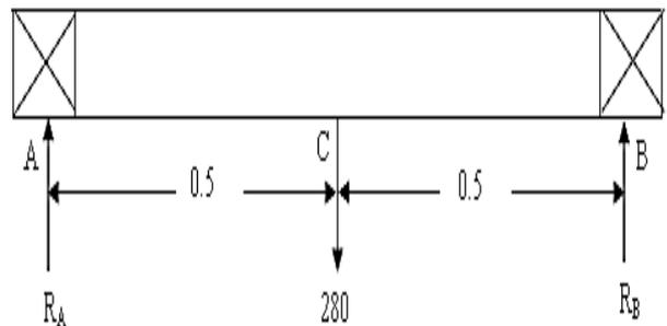
Fig. 19: Resolution of the Forces Acting On the Shaft of the Billboard
