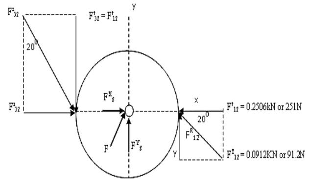
Fig. 14: Force diagram of the transmitted load on the gear assembly
