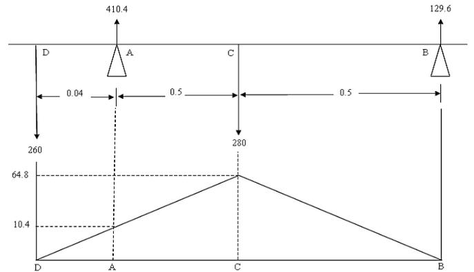
Fig. 18: The Bending Moment Diagram of the Forces Acting On the Shaft of the Billboard
