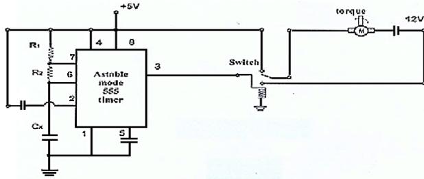
Fig. 4: The 555 timer circuit
