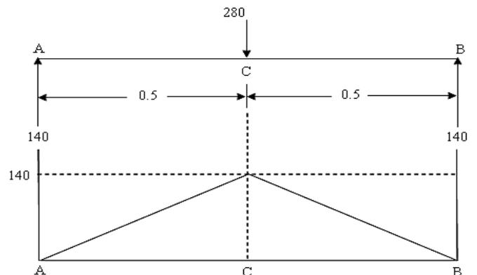
Fig. 20: The Bending Moment Diagram of the Forces Acting On the Shaft of the Billboard
