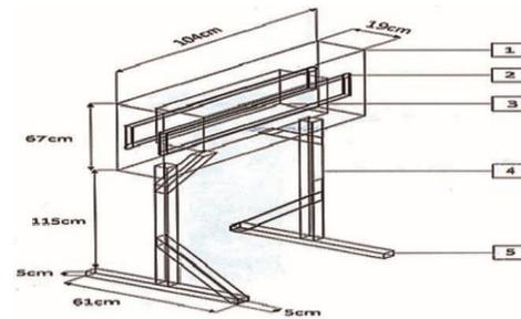
Fig. 1: An isometric view of the billboard (Assembling drawing)
