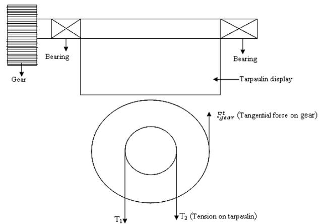
Fig. 15: Forces acting on the shaft members and housing
