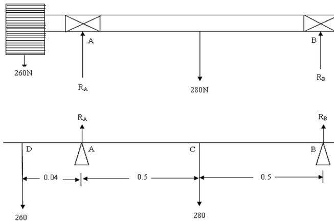
Fig. 17: Resolution of the Forces Acting On the Shaft of the Billboard
