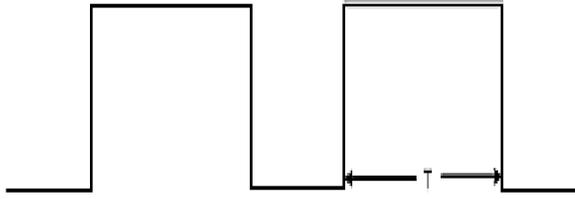
Fig. 7: The Waveform Configuration of a Monostable 555 Timer
