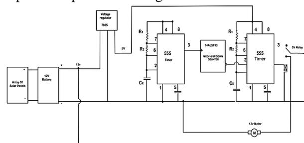
Fig. 3: The schematic diagram of the circuit and its integrated components for the supply of electricity and timing.
