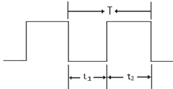
Fig. 6: The Waveform Configuration of an Astable Mode 555 Timer
