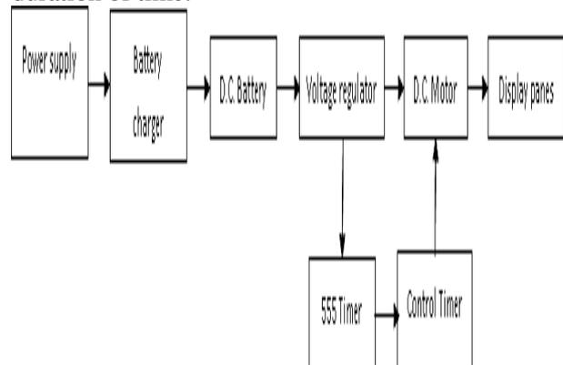
Fig. 2: Circuit for the supply of power
