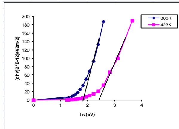
Fig. 3: A graph of  $(\alpha hv)^2$  versus  $hv$  for PbS thin film
