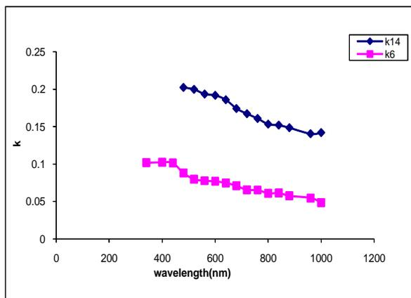
Fig. 4: A Graph of extinction coefficient versus wavelength for PbS thin film.
