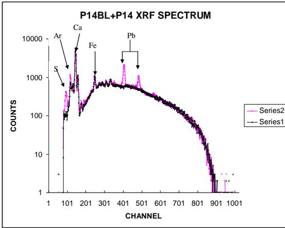
Fig. 1: Composition of lead sulphide sample (EDXRF)
