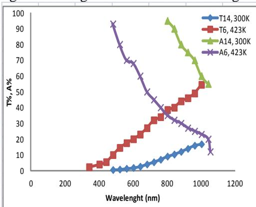
Fig. 2: A graph of percentage transmittance, T and absorbance, A versus wavelength for PbS thin films
