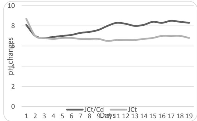
Fig. 3: pH Changes at Two Days Intervals for the Blended Waste Systems During Digestion Period
