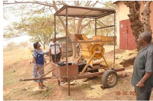
Fig. 1: Picture of the solar powered rice thresher mounted on a tractor-drawn trailer
